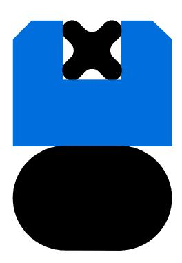
Very efficient double acting piston seal for reciprocating applications.
