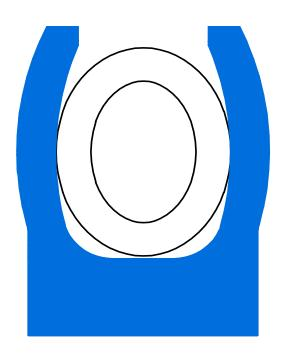
Spring energized flange seal for external pressure
