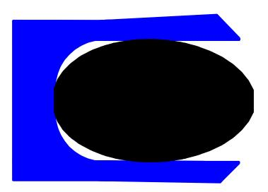
Single acting piston seal. For reciprocating and static applications.
