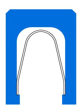
Spring energized flange seal for internal pressure
