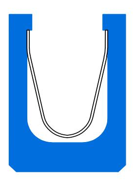
Spring energized flange seal for external pressure
