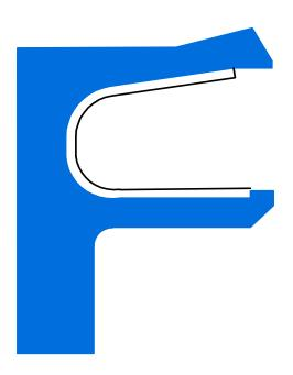
Spring energized Piston seal for rotating applications
