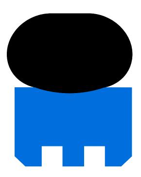
Rotating double acting seal for rods and shafts. Pressure up to 30 MPa.
