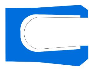
Spring energized rod seal for dynamic applications
