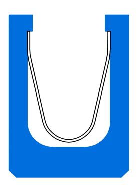
Spring energized flange seal for external pressure
