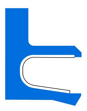
Spring energized rod seal for rotating applications
