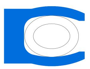
Spring energized piston seal for static applications
