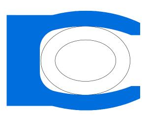
Spring energized piston seal for static applications
