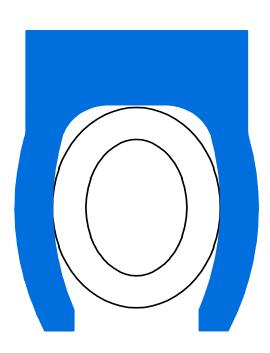
Spring energized flange seal for internal pressure
