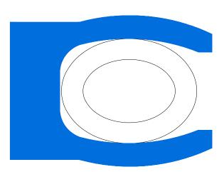
Spring energized rod seal for static applications
