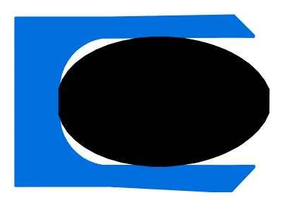
Single acting rod seal. For reciprocating and static applications.
