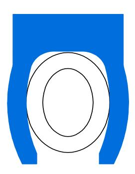
Spring energized flange seal for internal pressure
