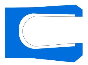
Spring energized rod seal for dynamic applications
