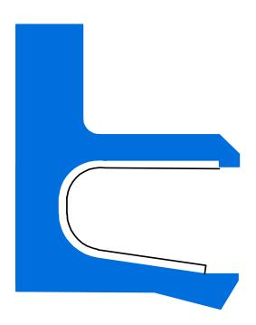
Spring energized rod seal for rotating applications
