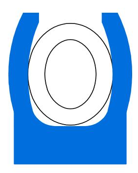
Spring energized flange seal for external pressure
