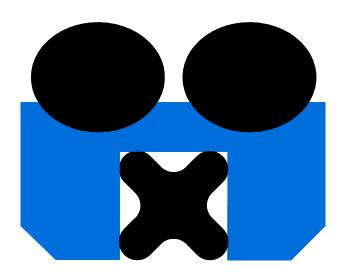
Very efficient double acting rod seal for reciprocating applications.
