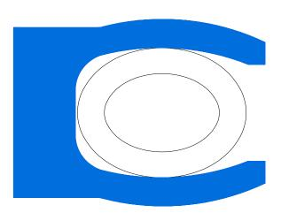
Spring energized rod seal for static applications
