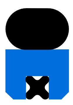
Very efficient double acting rod seal for reciprocating applications.
