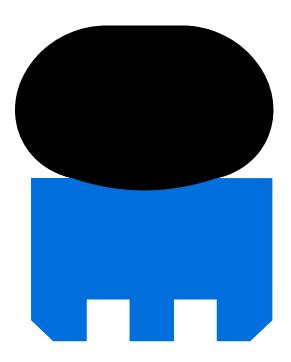
Rotating double acting seal for rods and shafts. Pressure up to 30 MPa.
