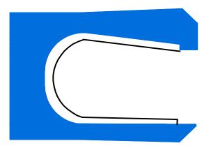
Spring energized piston seal for dynamic applications
