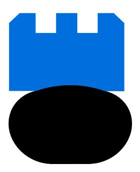
Rotating double acting seal for bore. Pressure up to 30 MPa.
