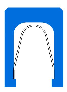
Spring energized flange seal for internal pressure
