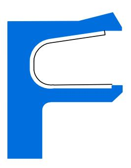
Spring energized Piston seal for rotating applications
